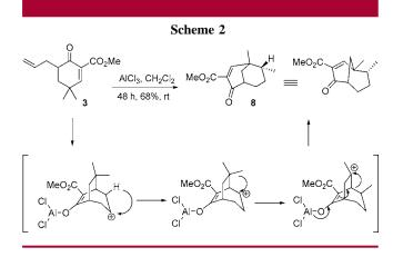
Following the formation of an aluminoxy complex, a cascade of  $\sigma$ -bond migrations comprising 1,2-hydride, 1,3-methyl, and 1,2-methine shifts is envisioned, culminating in the formation of the bicycle[3.3.1]nonane **8**.<sup>12</sup>
